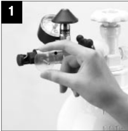
1 Feed curling ribbon through ribbon guide hole located under tying post. Place the balloon disc on tying post.
