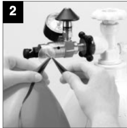
2 Hold the inflated balloon in your left hand. With your right hand, pinch the neck of the balloon and the ribbon together and stretch both around the end of the tying post.
