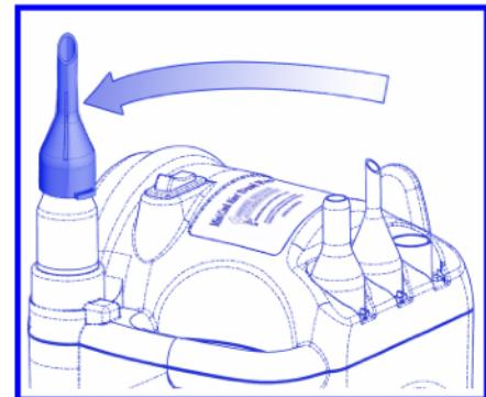
The Cool Aire® Nozzle has special grooves inside the nozzle that help reduce the inflation pressure even more and it also helps inflate with cooler air.
