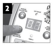
Set the Dual Split-Second Sizer to MODE 2 on the control panel. Reference the following chart to set the unit to properly inflate the balloons.
