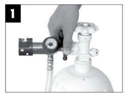
Hand-tighten the primary regulator to a helium or nitrogen cylinder. (For Italian and Russian inflators use a wrench to tighten regulator.) Make sure the cylinder is properly secured in a safety stand or wall bracket prior to attaching the primary regulator. **Do not open the cylinder valve until Step 6.**
