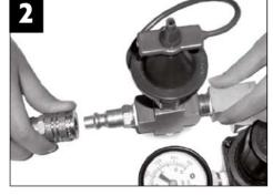
Push to connect the supply hose to the back outlet on the Dual Split-Second Sizer.
