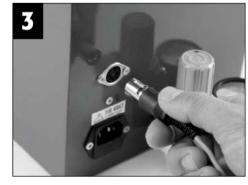
Plug the foot pedal into the back of the unit.
