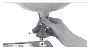
Place the foil balloon over the inflating outlet. Pinch the neck of the balloon between thumb and forefinger and press down on the outlet. Support the foil balloon in an upright position to insure the neck of the balloon does not fold over the outlet and restrict the flow of helium. When the balloon has reached the proper pressure the inflator will automatically shut off the helium flow. Remove the balloon from the outlet and attach a ribbon and a balloon weight.
