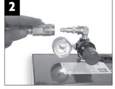
Connect the supply hose to the adjustable regulator in the back of the unit.
