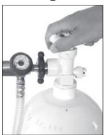
Close the cylinder valve or shut off the air compressor.
