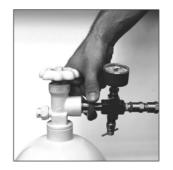
STEP 3. Remove the regulator assembly and replace cylinder. Hand-tighten the regulator assembly to the full helium cylinder. Close bleed valve.
