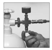
**STEP 2.** Open the bleed valve to release the pressure from the regulator assembly.
