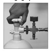
**STEP 1.** Close the cylinder valve tightly. Note: It is not necessary to close the valve on the Under Counterop Outlet.
