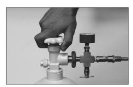
**STEP 4.** Slowly open the cylinder valve on the regulator assembly. Make sure the valve is fully opened. The cylinder pressure will read on the gauge located on the regulator assembly. The inlet pressure will read on the adjustable regulator gauge located ont he back of the inflator.
