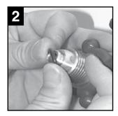
2. Use spray silicone to lubricate the new O-ring and press fit over tip of nipple into the groove.
