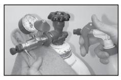
Connect inflator to a full cylinder. Slowly open valve and pressurize the inflator. Use a squirt bottle with a stream setting to apply a soapy-water mixture to each connection. Hold a rag behind the test area and spray a generous amount of the soapy water at the base of the connection. Bubbles will form in the water if the connection leaks.
