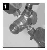
1. If the ribbon cutter is broken off completely, attach the inflator to a cylinder. Make sure the cylinder valve is closed and that there isn't pressure in the inflator.
