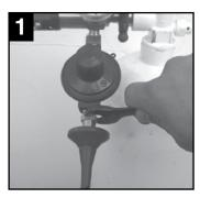
1. Attach the inflator to a cylinder; make sure the valve is closed and there is no pressure in the inflator. Rotate the regulator downward. Use a 5/8" open-end wrench to remove the Auto-Fill Foil Outlet.
