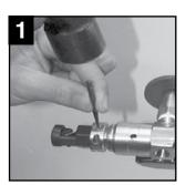
1. Attach the inflator to a cylinder; make sure the valve is closed and there is no pressure in the inflator. If the disc tyer post is broken off completely, drill a small pilot hole in the end of the broken disc tyer. Tap a easy-out bit into the pilot hole.
