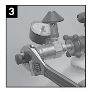
3. Use a wrench to lightly tighten the new ribbon cutter. Make sure to align the cutter with the blade pointing upward.
