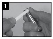
1. Hold the fitting between your thumb and forefinger. Place the Teflon tape on the second thread in from the end of the fitting first thread. Pinch the tape under your thumb and rotate the fitting counter clockwise. To apply a sufficient amount of tape rotate the fitting 3-4 full turns.
