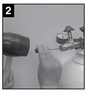
2. Use a rubber mallet to tap a small flat-head screwdriver into the remaining stub of the ribbon cutter. Carefully unscrew the broken end out of the ribbon cutter port.
