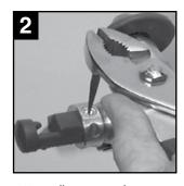
2. Use a plier to rotate the easy-out counter clockwise to remove the broken piece.
