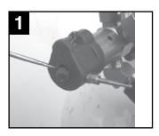
1. Attach the inflator to a cylinder. Make sure the cylinder valve is closed and that there isn't pressure in the inflator. Using a pick pry off the screw cap on the side of the ribbon cutter.
