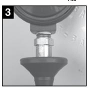
Leave approximately 2-3 threads exposed when tightening the new outlet or pressure gauge into the regulator. Leak check the connection under full pressure.
