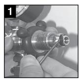
1. Remove the O-ring from the groove with a pick
